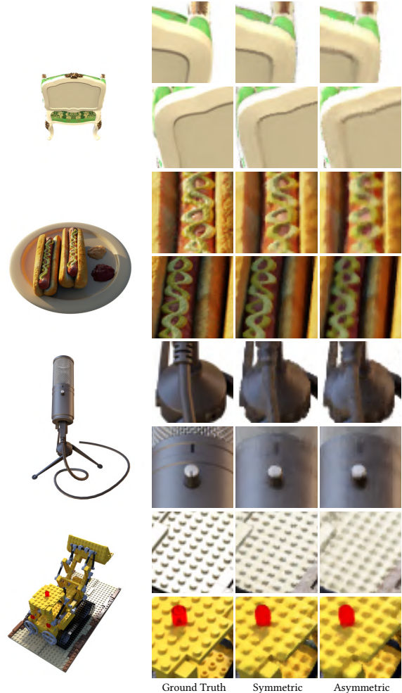
Figure 2: Visual results when both the downscale method and supervision signal are “average” (Input resolution is 100 \times 100 and upsampled by 4). Compared to asymmetric operation, symmetric averaged downscale and upscale produce more detailed super-resolution novel view synthesis.
