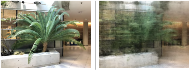
Figure 3: Mip-NeRF can synthesis reasonable novel views on trained resolution (left) but failed to generalize to higher resolutions (right).
