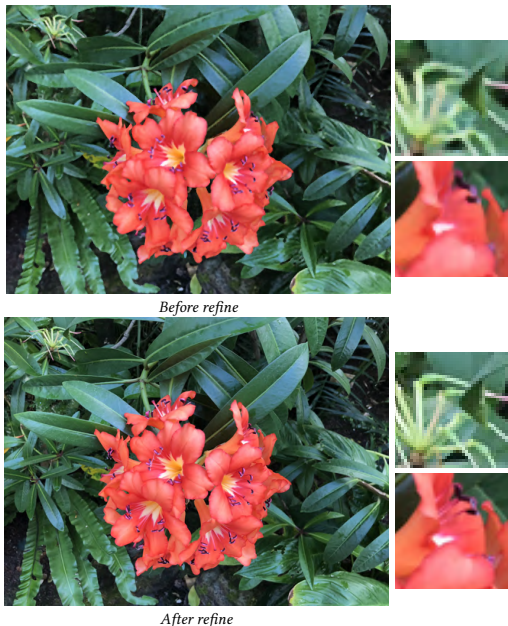
Figure 1: An example of refinement comparison for magnification of 2 for flower. Although the PSNR is decreased from 29.23 dB to 29.01 dB after refinement, see how it still improves visual quality.
